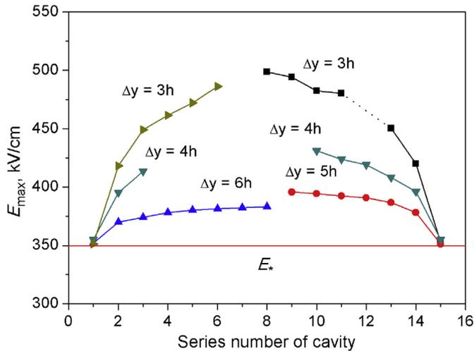
Fig. 8. The maximal values of electric field ahead of the front of the waves of PDs at different distances between cavities  $\Delta y$ .  $L = 1$  mm.  $h = 5 \mu\text{m}$   $E_* = 350$  kV/cm.  $\alpha = 20$  cm/(kV·ms). Lattice size is  $200 \times 200$ .
