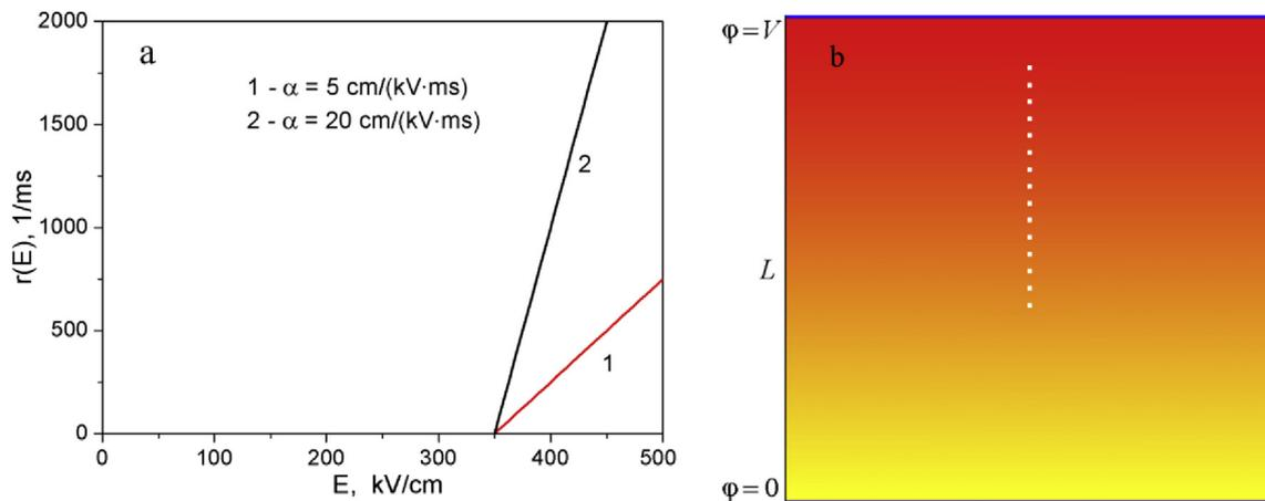
Fig. 1. (a) Probability function  $r(E)$  for PD in a cavity. Curves 1 and 2 correspond to  $\alpha = 5$  and  $20$  cm/(kV.ms). (b) Chain of gas cavities in the solid dielectric.  $N = 15$ .  $L = 1$  mm  $\Delta y = 6h$ .
