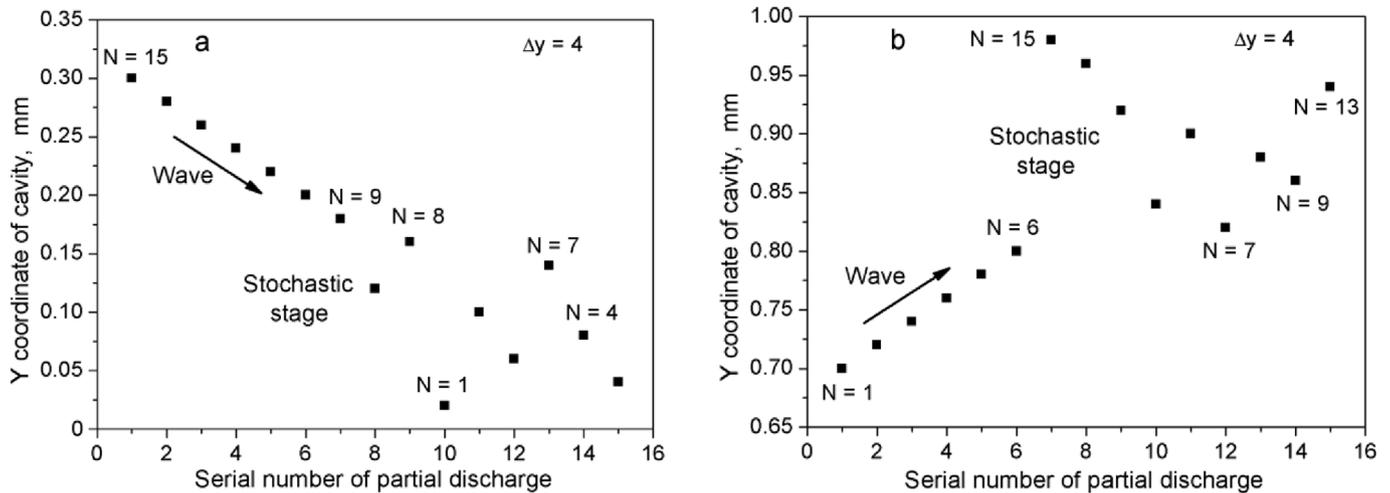
Fig. 10. The sequence of partial discharges in cavities. Wave of PDs and stochastic stage for the chains shifted down (a) and shifted up (b).  $L = 1$  mm.  $E_* = 350$  kV/cm.  $\Delta y = 4h$ .  $h = 5 \mu\text{m}$   $\alpha = 20$ (a) and 5(b) cm/(kV·ms). Lattice size is  $200 \times 200$ .
