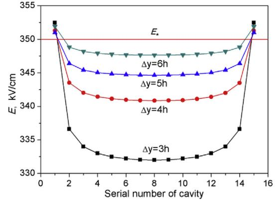
Fig. 5. The values of electric field inside all gas cavities just before the first partial discharges in the chain for different distances between cavities.  $L = 1$  mm.  $h=5 \mu\text{m}$   $\Delta y = 3h(2.8456$  ms),  $4h(2.7955$  ms),  $5h(2.7729$  ms),  $6h(2.7688$  ms).  $E_* = 350$  kV/cm.  $\alpha=20$  cm/(kV·ms). Lattice size is  $200 \times 200$ .
