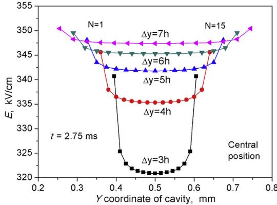
Fig. 3. The values of electric field inside gas cavities before the partial discharges ( $t=2.75$  ms) at different distances between cavities  $\Delta y = 3h, 4h, 5h, 6h, 7h$ .  $N = 15$ .  $L = 1$  mm.  $E_* = 350$  kV/cm.  $h=5 \mu\text{m}$   $\alpha=20$  cm/(kV·ms). Lattice size is  $200 \times 200$ .
