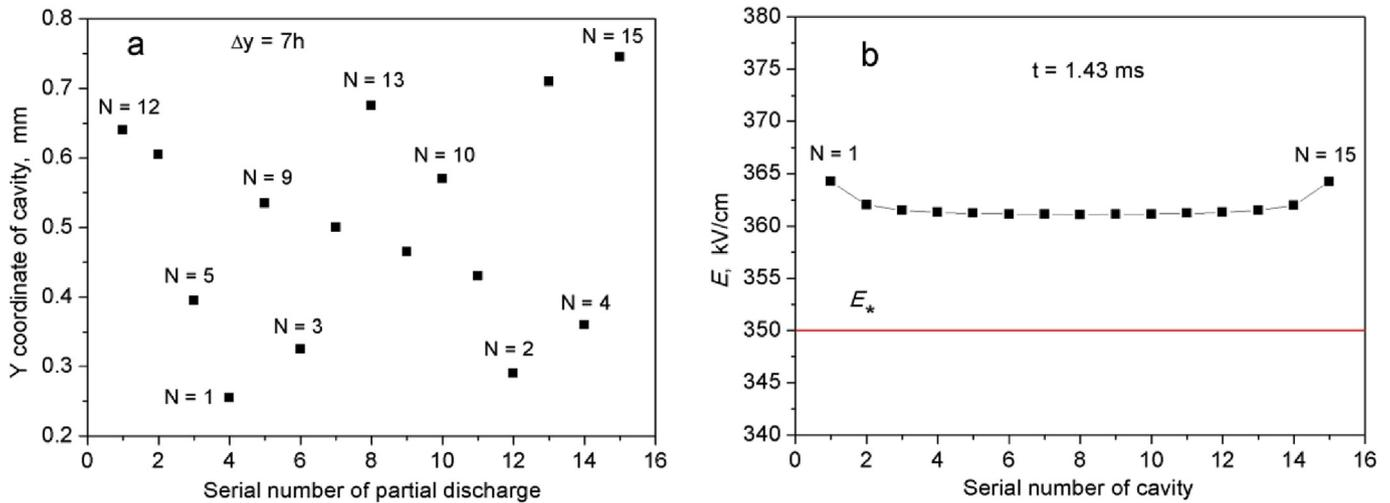
Fig. 9. (a) The stochastic regime of partial discharges in the chain of cavities. (b) The values of electric field inside cavities before the first PD ( $t = 1.43$ ms).  $L = 1$  mm.  $E_* = 350$  kV/cm.  $\gamma = 20$  kV/s.  $\Delta y = 7h$ .  $h = 5 \mu\text{m}$   $\alpha = 1$  cm/(kV·ms). Lattice size is  $200 \times 200$ .
