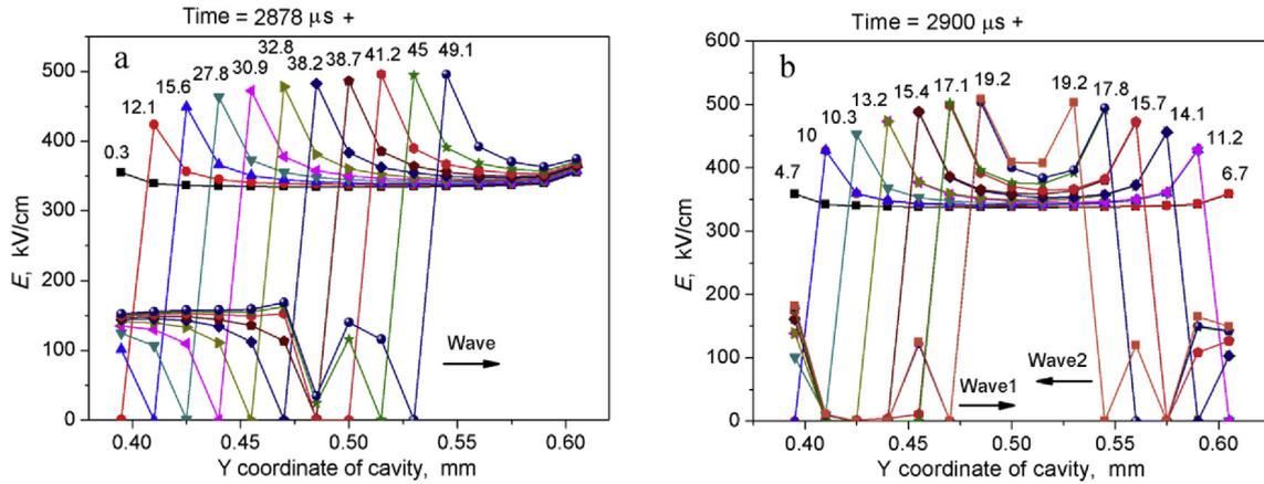
Fig. 7. The electric field values inside the cavities as the waves of PDs propagate along the chain. (a) One wave of PDs. (b) Two waves of PDs from the both edges of the chain.  $L = 1$  mm.  $E_* = 350$  kV/cm.  $\Delta y = 3h$ .  $h = 5 \mu\text{m}$   $\alpha = 1$  cm/(kV·ms). Lattice size is  $200 \times 200$ .
