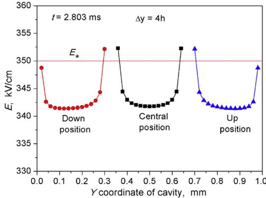
Fig. 4. The values of electric field inside gas cavities before the partial discharges ( $t=2.803$  ms) at different position of the chains ( $N = 15$ ).  $L = 1$  mm.  $E_* = 350$  kV/cm.  $\Delta y = 4h$ .  $h=5 \mu\text{m}$   $\alpha=20$  cm/(kV·ms). Lattice size is  $200 \times 200$ .
