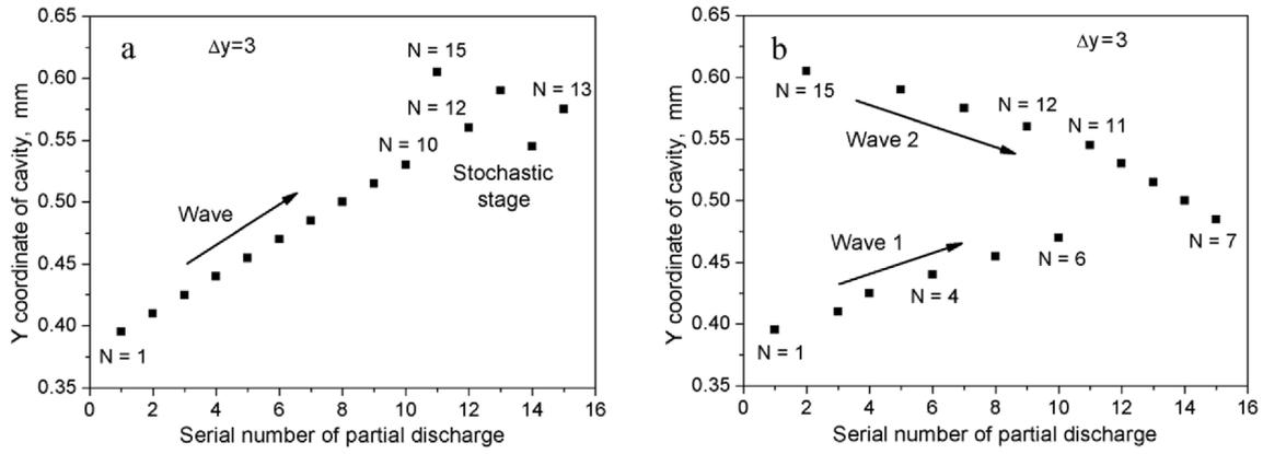
Fig. 6. The sequence of partial discharges in the cavities. (a) One wave of PDs and the stochastic stage. (b) Two waves of PDs from the both edges of the chain.  $L = 1$  mm.  $E_* = 350$  kV/cm.  $\Delta y = 3h$ .  $h = 5 \mu\text{m}$   $\alpha = 1$  cm/(kV·ms). Lattice size is  $200 \times 200$ .
