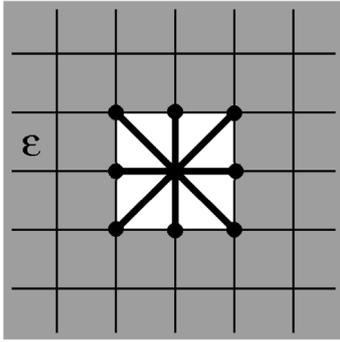
Fig. 2. The pattern of conductive structure arising in a cavity during a partial discharge that we used in simulations.
