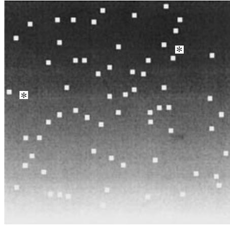
**Fig. 1.** The arrangement of voids in a typical variant of simulations. The potential varies from  $\varphi = 0$  at the bottom electrode to  $\varphi = V_0$  at the top electrode, as indicated by gray levels ( $N = 68$ ;  $100 \times 100$  grid).
