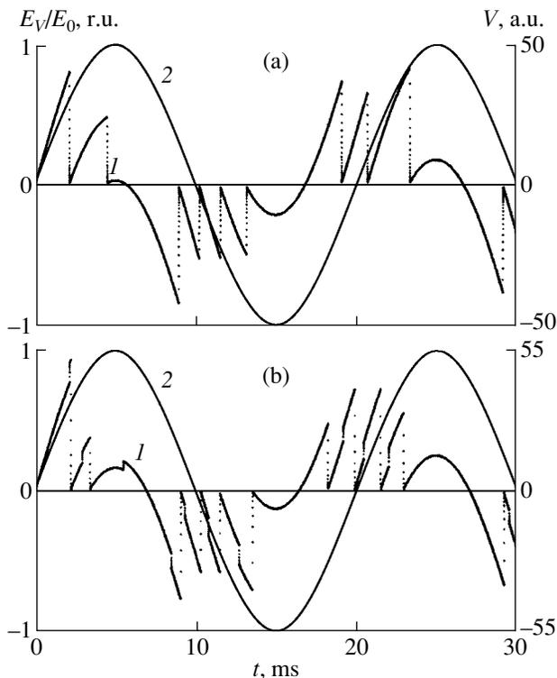
**Fig. 3.** Time variation of the applied voltage (curves 2) and the relative electric field strength (curves 1) (a) inside a single void occurring ( $V_0 = 50$ ) and (b) inside one of the two voids closely spaced in the direction along the field ( $V_0 = 55$ ) in a solid dielectric ( $\epsilon = 2$ ).
