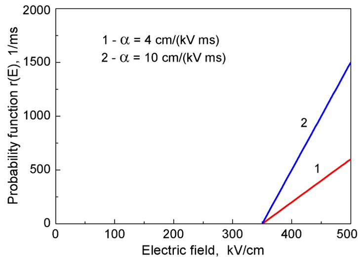
**Figure 2.** Probability function  $r(E)$  for PD in a cavity ( $d = 10 \mu\text{m}$ ).  $\alpha = 4$  (curve 1) and 10 (curve 2)  $\text{cm}/(\text{kV}\cdot\text{ms})$ .
