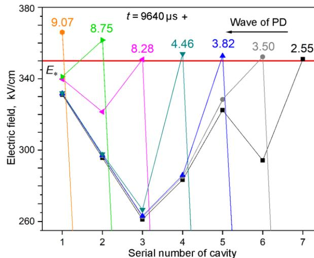
**Figure 5.** The magnitudes of electric field inside the cavities as the second wave of PDs propagates along the chain of caverns from right to left (series 2 in Figure 3).
