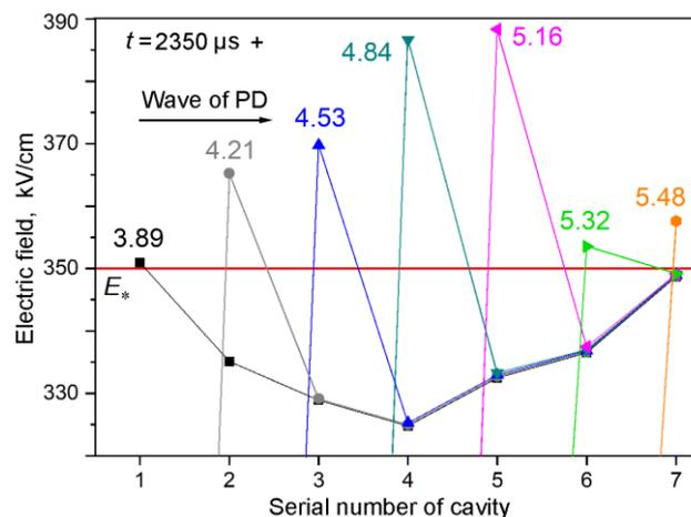
**Figure 4.** The magnitudes of electric field inside the caverns as the first wave of PDs propagates from left to right along the chain (series 1 in Figure 3).  $L = 0.256 \text{ mm}$ .  $E_* = 350 \text{ kV/cm}$ . Lattice size is  $1024 \times 1024$ .
