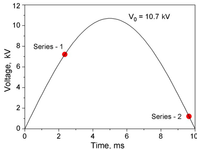
**Figure 3.** The value of applied AC voltage vs. time. Two series of partial discharges in the chain.
