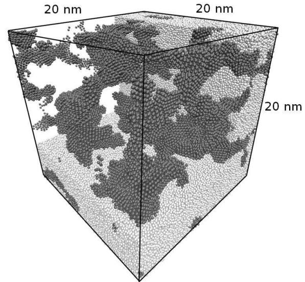
**Figure 1.** Simulation of the carbon condensation in DP. The light balls are the DP molecules, the dark balls are the carbon atoms. The volume fraction of the carbon atoms was 10 percents. Only the carbon component is shown in the part of the simulation region for clarity.
