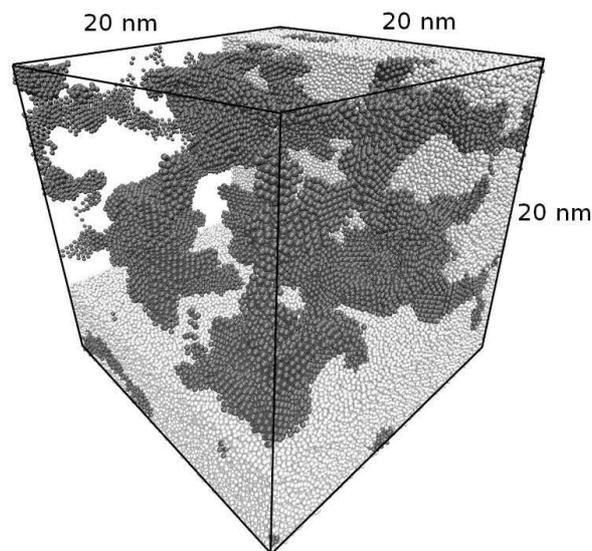
**Figure 1.** Simulation of the carbon condensation in DP. The light balls are the DP molecules, the dark balls are the carbon atoms. The volume fraction of the carbon atoms was 10 percents. Only the carbon component is shown in the part of the simulation region for clarity.
