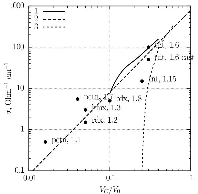
**Figure 3.** Electrical conductivity of detonation products. 1—electrical conductivity of carbon nets simulated using MD, 2— $\sigma_0 (V_C/V_0)^2$ , 3—percolation model, points are the experimental data for different HE.
