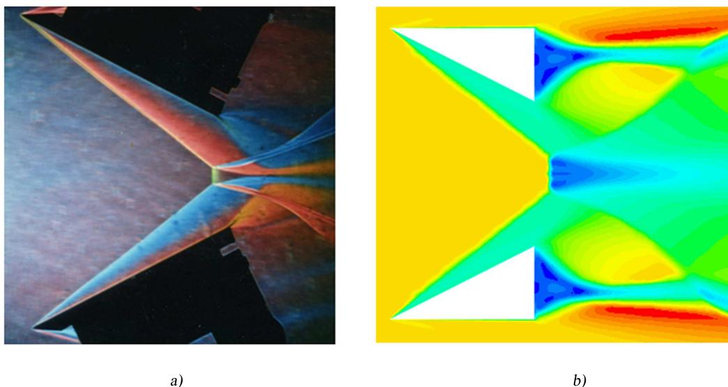
**Figure 7.** Shlieren picture (a) and numerical solution (b) of three shock configuration in air, vertex angle of wedge equals 27 deg.. Mach number equals 5.
