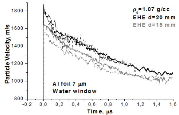
**Figure 1.** Particle velocity profiles of 7  $\mu\text{m}$  Al foil situated between an explosive charge and a water window obtained in VISAR experiments with EHE. Grey profiles are for 15 mm diameter charges; black profiles are for 20 mm diameter charges.
