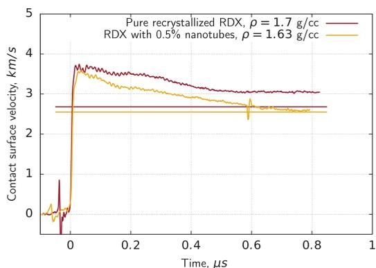
Fig. 7. Velocity of contact boundary HEs – PMMA. The horizontal lines show the calculated velocity levels for the Chapman-Jouguet state.
