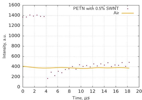
Fig. 9. Integral SAXS during detonation of PETN-based composite.
