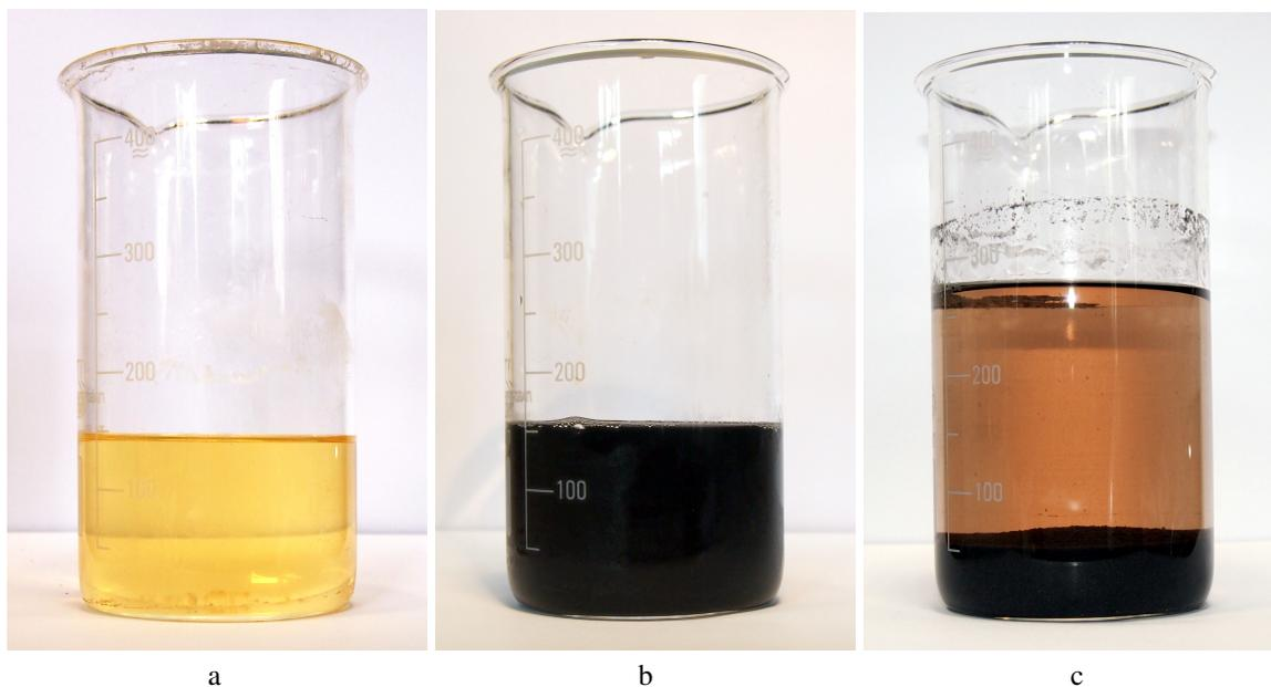
Fig. 1. TNT+0.5% wt SWCNTs synthesis, a – solution of TNT in acetone, b – SWCNTs dispersed in water, c – precipitated explosive composite.
