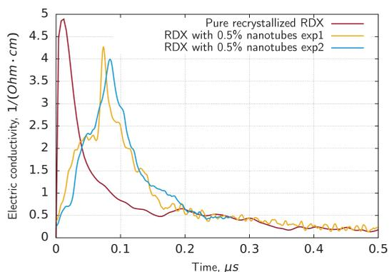
Fig. 6. Electrical conductivity behind the detonation front for a pure RDX and a composite. The charge density in all cases is  $1.8 \text{ g/cc}$ .
