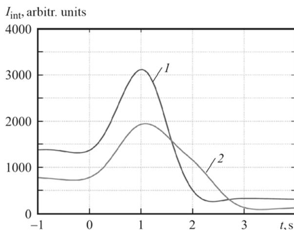
Fig. 3. Experimental dependences of the integral radiation intensity on time in combustion of compounds with boron (1) and aluminum-dodecaboride additives (2).
