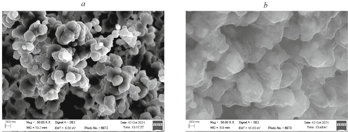
Fig. 4. EM images of the original particles of the additive of boron (a) and the products of its combustion (b).
