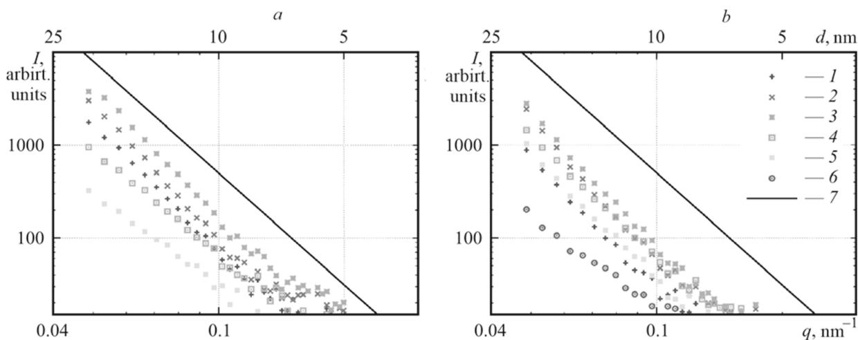
Fig. 2. Experimental dependences of the intensity of radiation from the combustion of the compound with boron (a) and aluminum-dodecaboride additives (b) on the scattering vector at the instants of time  $t = 0$  (1), 0.5 (2), 1.0 (3), 1.5 (4), 2.0 (5), and 2.3 s (6): 7)  $q^{-4}$ .
