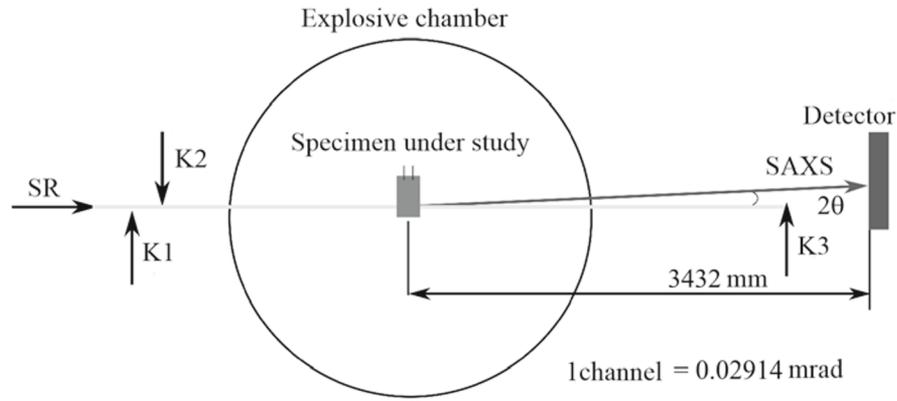
Fig. 1. Scheme of experiments on measuring small-angle x-ray scattering.
