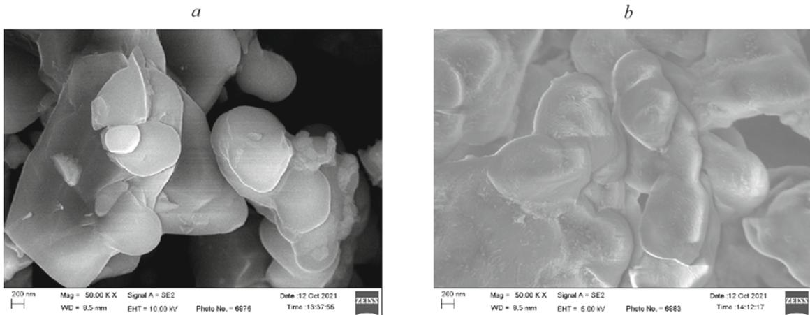
Fig. 5. EM images of the original particles of the additive of aluminum dodecaboride (a) and the products of its combustion (b).
