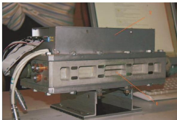
Fig. 3. General view and properties of x-ray detector DIMEX-3. 1 – entrance slit, 2 – electronic block. Strip size – 100 mkm, number of space channels – 512, number of time frames – 32, shortest exposition – 125 ns.
